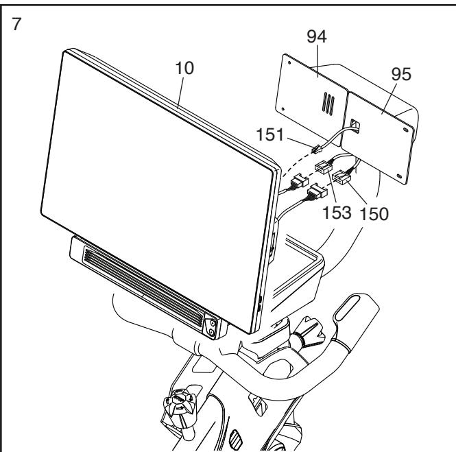
8. **Tip: Avoid pinching the wires and the cable. If necessary, tilt the Left and Right Console Brackets (94, 95) to make this step easier.**
