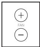
Note: If the pedals are not moved for a while when the main menu is selected, the fan will turn off automatically.
