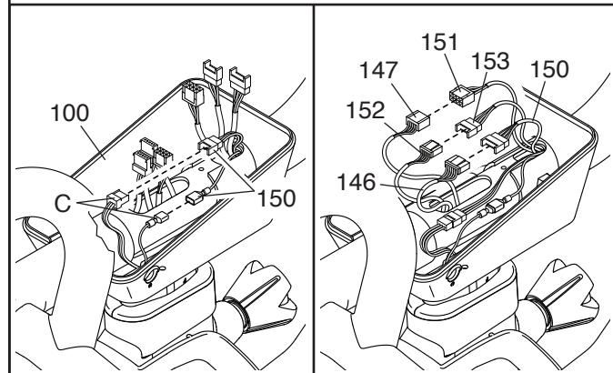
6. **Tip: Avoid pinching the wires and the cables.** Set the Accessory Tray (99) on the Tray Base (100). Attach the Accessory Tray to the Handlebar Post (7) with four M4 x 20mm Machine Screws (9) (only two are shown); **start all four Machine Screws, and then tighten them.**
