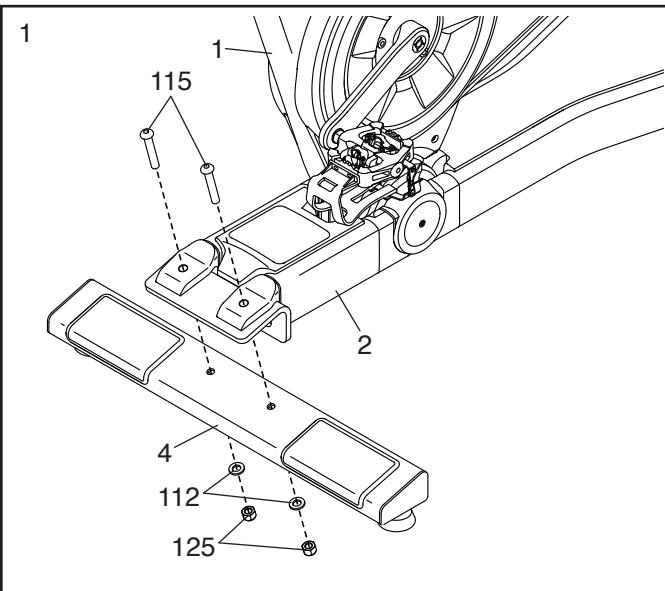
2. Set a sturdy piece of packing material under the front of the Base (2). **Have a second person hold the Frame (1) to prevent it from tipping while you complete this step.**
