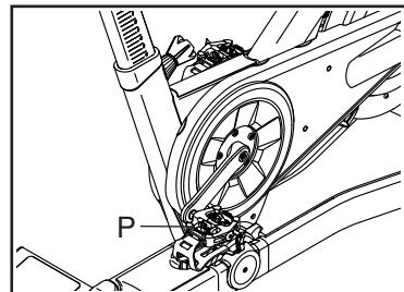
To use the clip-in side of the pedals, you must wear cycling shoes. To clip into the pedals, press the cleats on your cycling shoes firmly into the slots in the pedals until they snap into place. To unclip from the pedals, twist your cycling shoes outward from the pedals.
