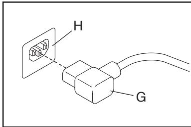
2. Plug the power cord (G) into an appropriate outlet (I) that is properly installed and earthed in accordance with all local codes and ordinances.
